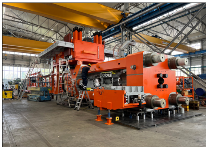
Figure 6. Jimi, the new extrusion press, as it was being constructed at the Danieli Breda plant in Italy.
