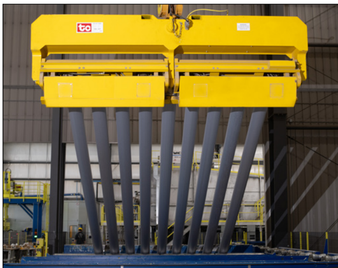
Figure 4. Hydraulic tongs remove 325 inch logs from the cast pit and lay them down on the conveyor table.
