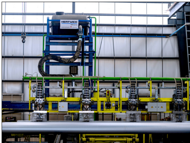
Figure 5. The quality of each billet is ensured using helical ultrasonic inspection station.
