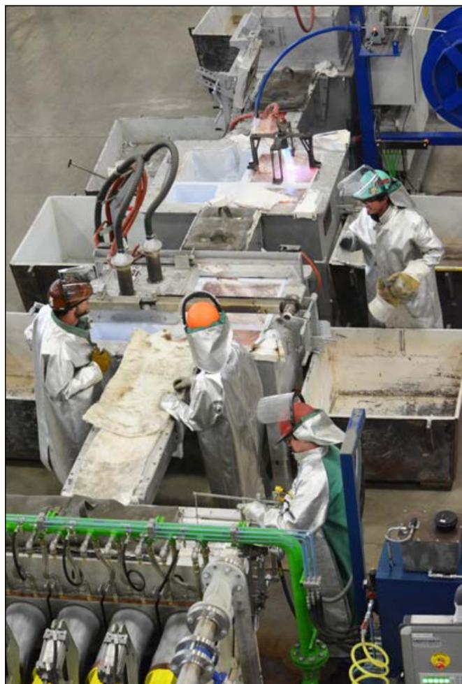
Figure 3. Casting initiated at the new CRP horizontal casting line.
