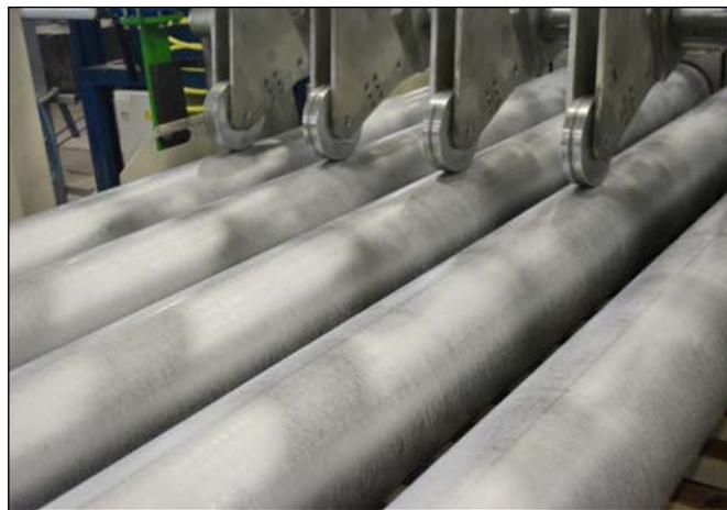
Figure 5. Close-up of LaserLog production from the horizontal casting mold, showing the typically smooth surface.
