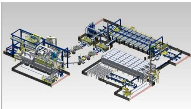
Figure 2. Layout of the Phase 2 CRP, which is similar in principle to Phase 1 in providing continuous material flow from scrap melting to log/billet bundling.
