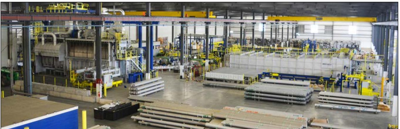
Figure 1. The Phase 2 CRP, with the melting furnace in the foreground (left), horizontal casting lines behind (center), and continuous homogenization furnace (right).
